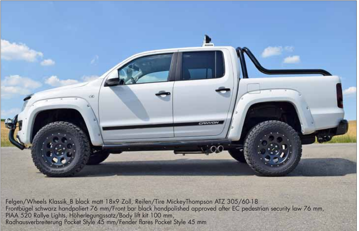
Frontbügel schwarz 76 mm/Front bar black approved after EC pedestrian security law 76 mm, PIAA 520 Rallye Lights, Schnorchel/Snorkel, Winde/Winch
